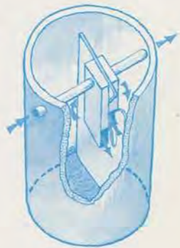
Septic tanks may be constructed of glass fibre, thermoplastics or precast concrete.
